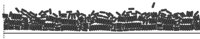
FIG. 2. Simulations 4: Rearrangement after 1200 s of vibrations. Initially the particles were ordered horizontally. Lateral walls are periodic.
